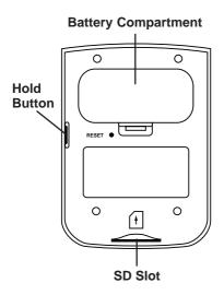
SD Slot: Insert an SD card here. Slide the SD card into the slot with the contacts facing the back of the device. Push gently until it clicks into place. To remove an SD card from the slot, put your thumb on the SD card and push it in slightly. You hear a click and the SD card pops out. Slide it out of the slot.
