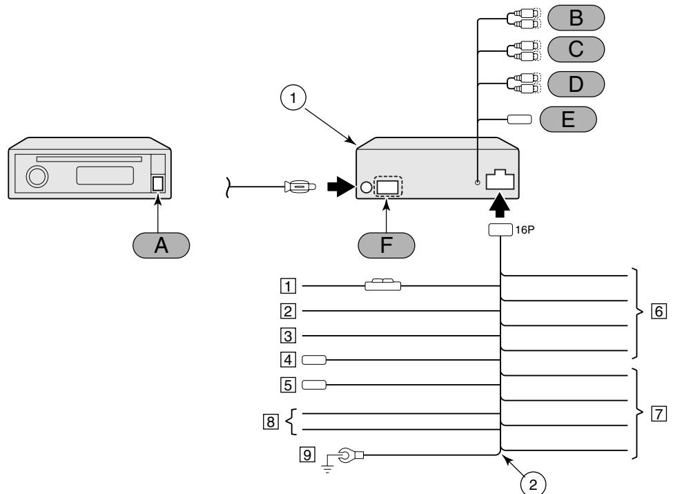
◆ Wire colors and connection points for connection wires ②
