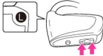
Adjust the volume with the VOL+/- button. The volume can be adjusted in 31 steps: from 0 to 30. "10" is set by default.
