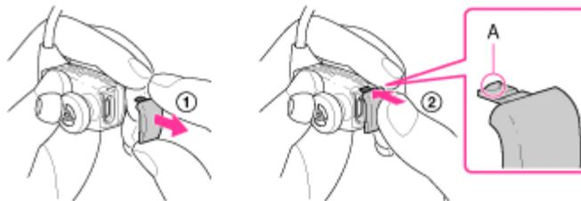
If the USB jack cover comes off, you can put it back on by pushing it back into the same position as that shown in the right figure (②).
