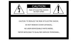
This symbol is intended to alert the user to the presence of uninsulated "dangerous voltage" within the product's enclosure that may be of sufficient magnitude to constitute a risk of electric shock to persons.
