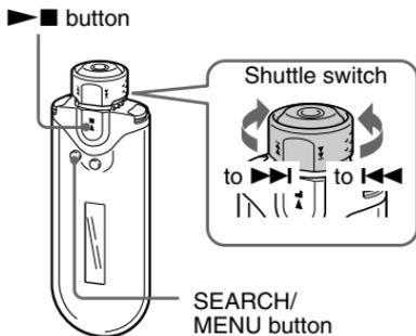
“Complete” is displayed when presetting is complete. Then, press the SEARCH/MENU button repeatedly to exit menu mode; the first preset station will be received.
