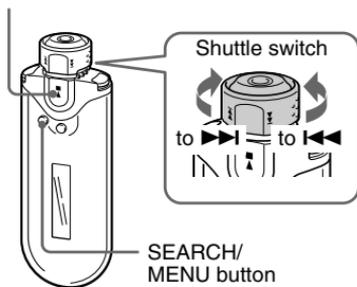
**2** Rotate the Shuttle switch to select “Sound>” and press the ▶■ button to confirm.
