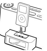
Adjust the rear support forward or backward checking the back of the iPod fits snugly against the rear support to protect the conn
