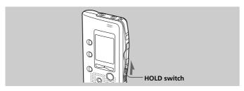
Slide the HOLD switch in the direction of the arrow. "HOLD" will flash three times, indicating that all the functions of the buttons are locked.
