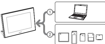
As shown on the left, the photo frame gives priority to the connection with computer if computer and memory cards are connected/inserted to the photo frame. If multiple memory cards are inserted, the images of the memory card you inserted first are displayed.
