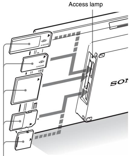
Insert a memory card firmly into the corresponding slot with its label side facing toward you. The slot order from the top is "Memory Stick" ("Memory Stick Duo"), CompactFlash card, SD memory card and xD-Picture Card.
