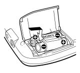
**3** Connect the AC power adaptor. The indication "CHG" lights up and the 'number 1" shifts position in succession until the battery is fully charged. Charging time is about 2 hours for BP DM10 and 3.5 hours for BP-DM20.
