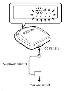
**4** When fully charged, "CHG" disappears. Disconnect the AC power adaptor
