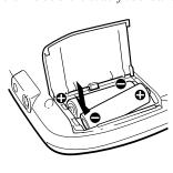
When to replace the dry batteries When the battery becomes weak, i indication flashes in the display. If the "Lo batt" appears in the display, replace all the batteries with new ones, because the batteries are used up.
