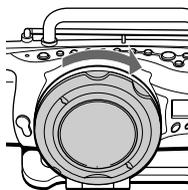
Close the lid of the CD compartment and turn it clockwise until the ● mark on the player and the ● mark on the lid align.
