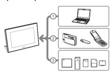
As shown on the left, the photo frame gives priority in order of computer, external device, and memory card if computer and memory cards are connected/inserted to the photo frame. If multiple memory cards are inserted, the images of the memory card you inserted first are displayed.
