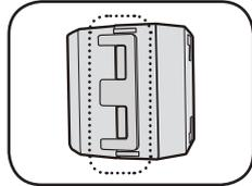
Lift up to release the lock and open the core.
