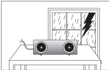
During thunderstorms, disconnect the AC plug from the wall outlet. Voltage peaks due to lightning could damage the unit.
