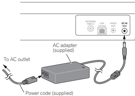
**1 Plug the supplied AC adapter into the DC IN socket on the back of the unit.**
