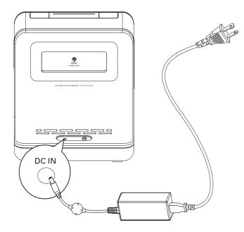
**3** Connect the other end of the AC adaptor to the wall outlet.
