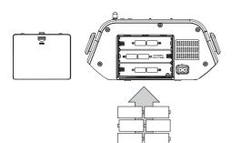
The unit can also be powered by batteries. (Requires 6 C size batteries, not included.
