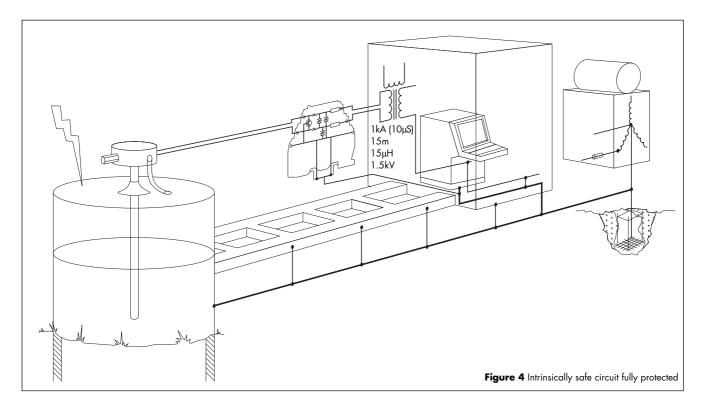
The system should be designed so that when the surge current is diverted the voltage drop across the bonding conductor does not create a large voltage across the isolator. Figure 4 gives an illustration of a satisfactory system. With the currents and distances indicated the isolator is still subjected to a 1.5kV pulse and hence the importance of keeping the interconnection as short as possible cannot be over emphasised.
