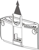
3.) Press on the bottom of the iPod® adapter as shown to remove it from the docking cradle.
