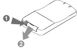
Install a fresh CR2032 battery in the holder as shown and slide the holder back in to the remote control.
