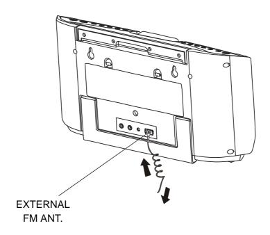
It may be necessary to adjust the direction of the FM antenna wire until you find the position that provides the best reception.
