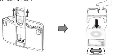
3. Choose the appropriate adapter for your particular iPod® model from among the 6 adapters supplied with this system and insert the adapter into the docking cradle as shown. (Refer to the iPod adapter chart).
