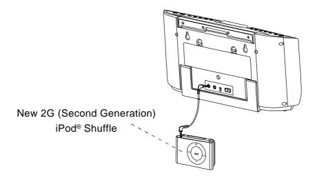
1.) Connect the headphone jack or Line Out jack of your external audio source to the **AUX IN** In jack on the back panel of this system.
