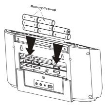
3.) Replace the battery compartment and make sure that it locks securely in place.
