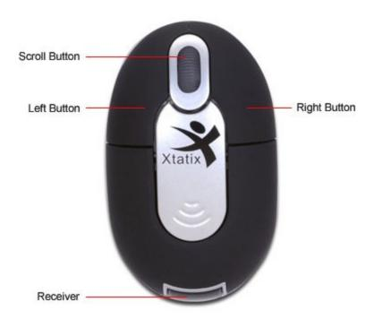
To put batteries in the mouse, pop off the black cover where your palm rests. The batteries go in there. The mouse requires two AAA batteries.
