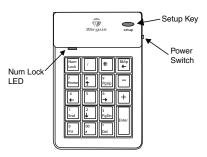
3 Turn on the keypad by sliding the Power switch on the right side of the keypad to the "on" position.
