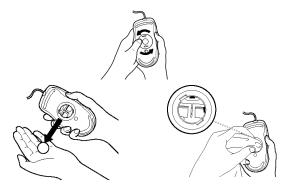
Figure 4. Removing and cleaning the mouse ball
