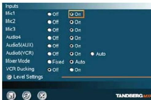
4. Adjust the audio Input Type Level if necessary (recommend +8dB)
