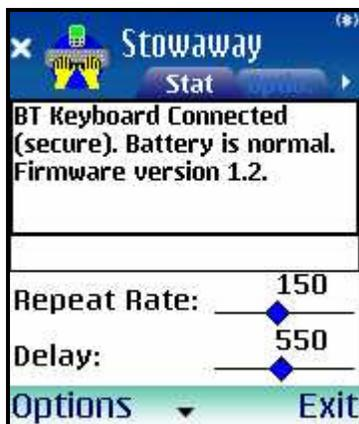
2. When the Bluetooth keyboard is enabled, the Status window shows the connection status, the battery state, and firmware version for the keyboard. The three states of the battery are:
