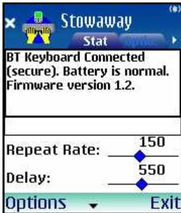
6. If the *Passkey* is entered successfully on both devices, the message **BT Keyboard Connected** will appear on the *Status tab*. If the keyboard does not show up as connected:
