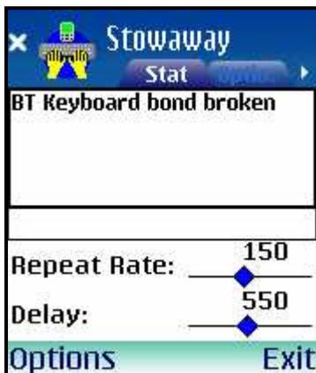
**NOTE:** Do not press <Ctrl> <Left Fn> <Right Fn> together. This will break the bond between the keyboard and the mobile device. If this happens, you will have to establish a new connection as described above.
