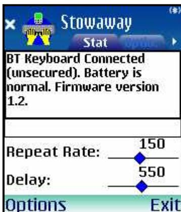
1. If you chose an *Unsecured* connection by selecting **Off** at the *Options tab > Bluetooth security* option, connection is usually established within a few seconds after pressing <Ctrl> <Left Fn> <Right Fn>. If the connection is not completed, press the <Ctrl> <Left Fn> <Right Fn> keys together again.
