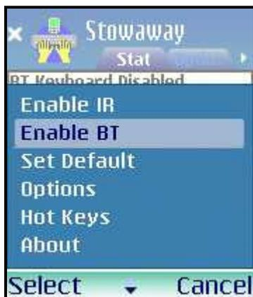
2. Press the left Softkey below **Options** to open the menu with selections to enable or disable the keyboard. This menu also gives access to the remaining application tabs. To enable the **Stowaway keyboard**, make sure the keyboard is **Discoverable** by the mobile device. Press the **<Ctrl> <Left Fn> <Right Fn>** keys together until the green LED (above the **<T>** key) flashes once per second.
