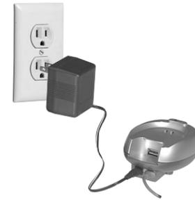
**Caution:** You must use a regulated Class II power source that supplies 5V DC and delivers at least 450 mA. Its center tip must be set to positive and its plug must fit the charger's DC jack. The supplied AC adapter meets these specifications. Using an adapter that does not meet these specifications could damage the charger or the adapter.
