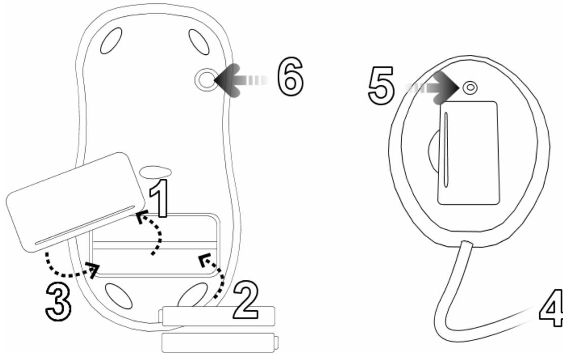
1. Remove the **Battery Compartment Cover** on the back of your Mouse.
