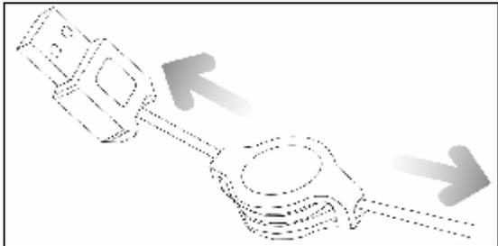
2. To retract the retractable USB cable, pull both ends of the cable by approximately ½" to unlock the cable and slowly retract it back into the cable retractor.
