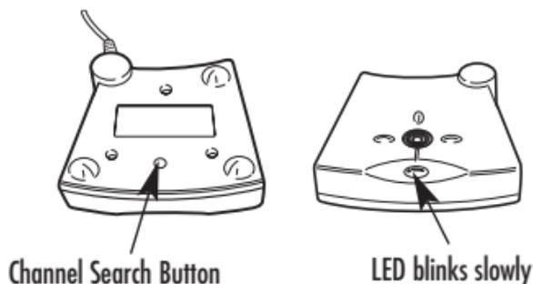
1. Press the Channel Search Button on the bottom of the receiver, and note the index LED will blink slowly.
