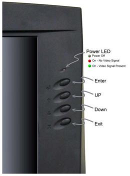
The first selection is the Auto Adjust function. Selecting this option brings up the Auto Adjust menu. Here you can select No or Yes using the up and down buttons. If you select Yes, the TFT will attempt to automatically detect your video output specifications and reset the TFT to match.
