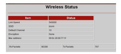
The Wireless Status Report shows you the modem speed (Link Speed), the SSID, your Default Channel, the Mac address of the modem, and the number of packets that are being received and transmitted (Rx and Tx Packets). You can also tell if your modem has wireless encryption enabled. (To encrypt your information, click the Wireless icon in the Zoom Configuration Manager).
