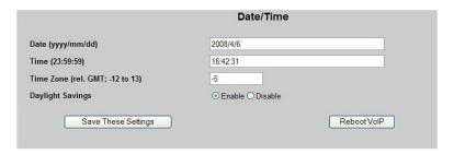
The date and time are set automatically by the time server, and the Daylight Savings adjustment is enabled by default.
