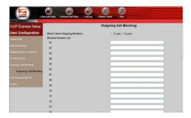
At the **Block Listed Outgoing Numbers** option, select the **Enable** check box. In the **Blocked Call List**, enter up to 30 complete numbers or numbers starting with particular digits. For example, to block all 900 numbers, enter 900x.7. This will block all numbers that start with 900 followed by 7 digits.
