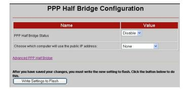
To configure a half bridge, set the Half Bridge status to **Enable**. From the drop-down list, choose the computer that you want to share the public IP address. This default setup for the PPP Half Bridge works for most applications. You should not need to make additional changes using the **Advanced PPP Half Bridge**.
