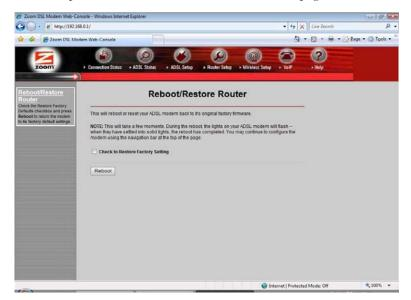
Click the **Check to Restore Factory Settings** check box, click **Reboot**, then follow the instructions to reset your ADSL modem to its original firmware. Please see **Backing Up and Restoring Your Configurations** on page 137 for information about restoring a stored X6v configuration.
