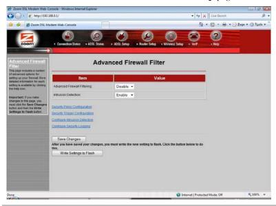
Important! Do not enable Advanced Firewall Filtering on the Advanced Firewall Filter page until you create your security policy. Otherwise, if you enable Advanced Firewall Filtering before you create your policy, you will block all outgoing and incoming traffic.
