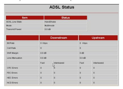
The **ADSL Line State** tells you where your modem is in the connection process. The three states are **Training**, **Handshake**, and **ShowTime**. A line state of **ShowTime** shows that your modem has established a physical connection to the DSLAM (DSL Access Multiplexer – a device used in the process of connecting your computers, and/or network to the Internet). **Training** is at the beginning of the connection and **Handshake** is right after **Training**.
