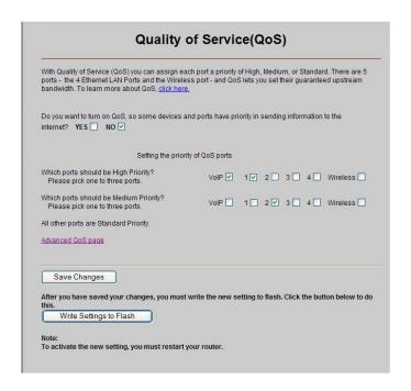
Note that on the QoS screen, Port 1 is the Ethernet port labeled ETHERNET 1 on the X6v back panel. Port 2 is ETHERNET 2, and so forth.
