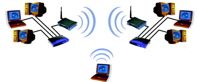
Figure 2-3: Network Using Wireless Bridging
