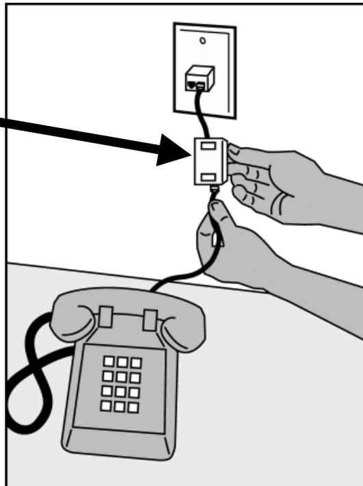
**5) Connect the data cable that will go to your DSL modem to the unfiltered side of the 2-way adapter**
