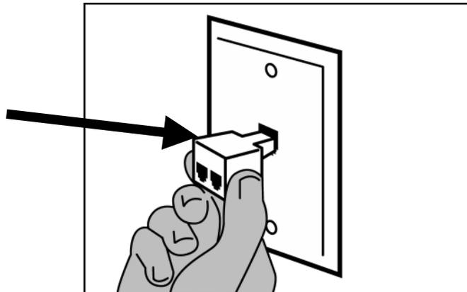
**3) Connect a filter to one side of the 2-way adapter**
