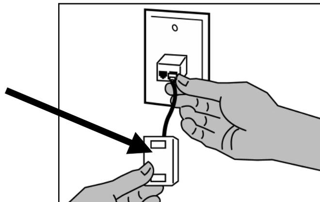
**4) If you have a phone, fax machine, analog modem or other phone device at this location, connect it to the filter**
