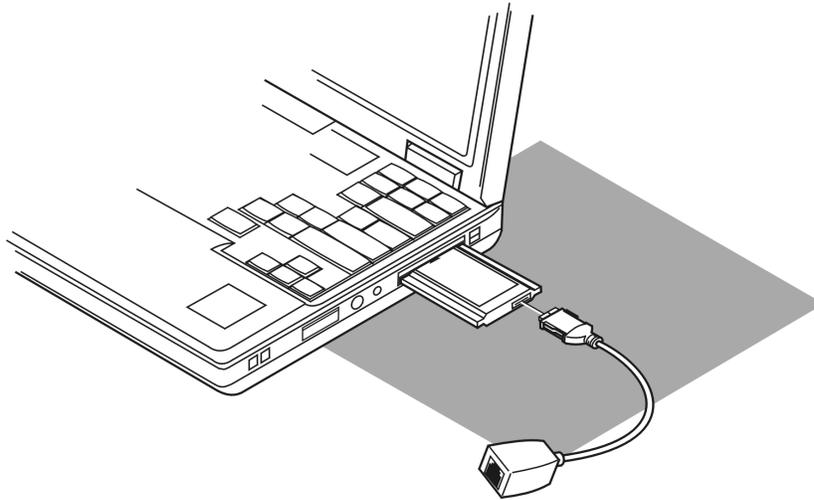
B-12 Carefully push the Media Access Module (MAM) into the socket on the Card until the locking tabs click into place.
