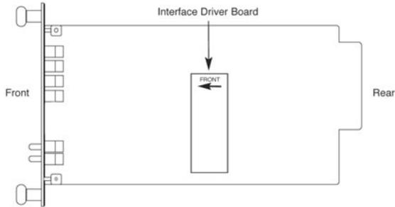
**Figure 7.** Driver Board mounted on Model 3088RC
