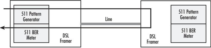
Figure 20. Remote Digital Loopback Diagram
