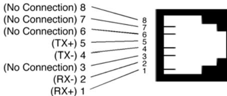
Figure 5. 120 ohm RJ-48C G.703/G.704 Interface
