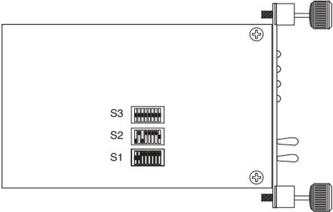
Figure 1. Location of DIP switches on Model 3088RC
