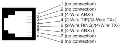
**Figure 10.** RJ-45 Line Interface
