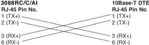
**Connecting the Line Interface.** The Model 3088RC/C/AI is to be used with Patton function card access products (i.e. 1092ARC) There are two essential requirements for connecting the line interface on Model 3088RC/C/AI:
