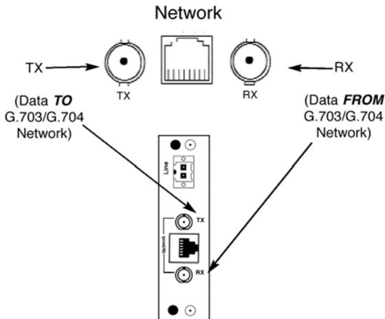
**Figure 6.** 75 ohm Dual Coaxial G.703 Interface
