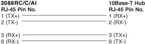
**Connecting the 10Base-T Ethernet Port to a PC (DTE).** The Model 3088RC/C/AI 10Base-T interface is configured as DTE (Data Terminal Equipment). If you wish to connect the 3088RC/C/AI to another DTE device such as a 10Base-T network interface card in a PC, you must construct a 10Base-T crossover cable as shown in the diagram below.
