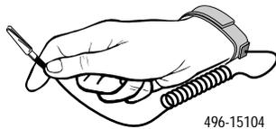
**This product is designed to protect sensitive components from damage due to electrostatic discharge (ESD) during normal operation. When performing installation procedures, however, take proper static control precautions to prevent damage to equipment. If you are not sure of the proper static control precautions, contact your nearest sales or service representative.**
