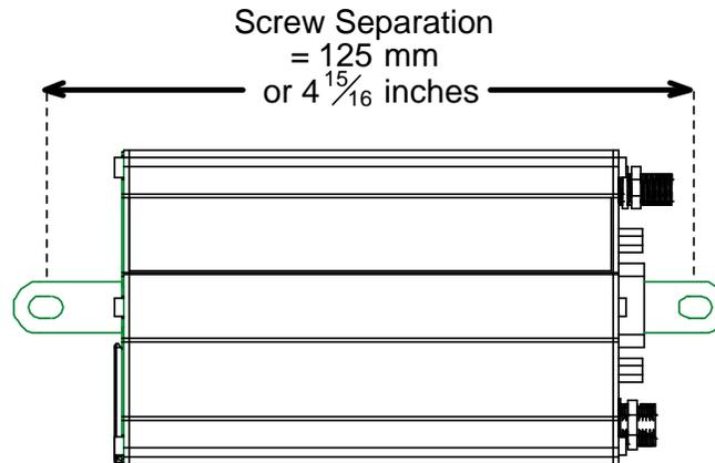
3. Slide the mounting bridles into the corresponding slots on the backside of the modem chassis.
