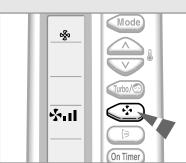
3 Select the fan speed by pressing the button one or more times until the required setting is displayed:
