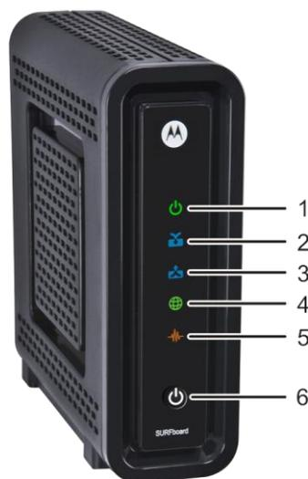
The SB6121 front panel icons provide the following modem status information for power, communications, and errors:
