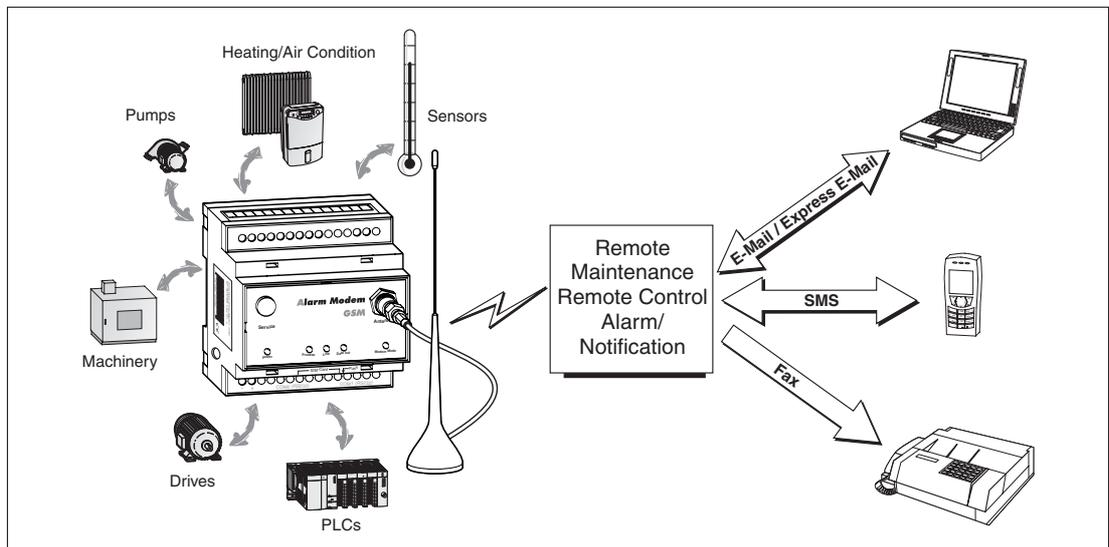
**Fig.1-1** Communicating possibilities with the Mitsubishi Alarm Modem
