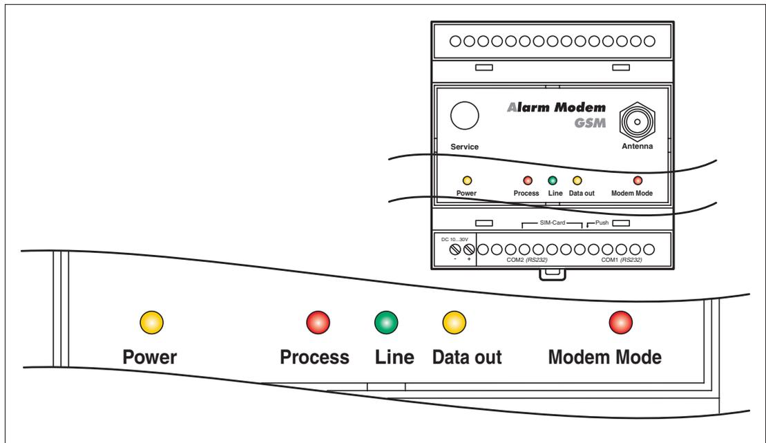
Fig. 6-1: LEDs on modem
