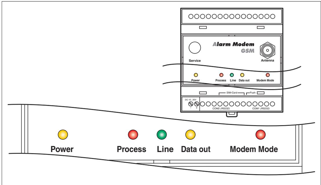
Fig. 3-3: LEDs on the modem
