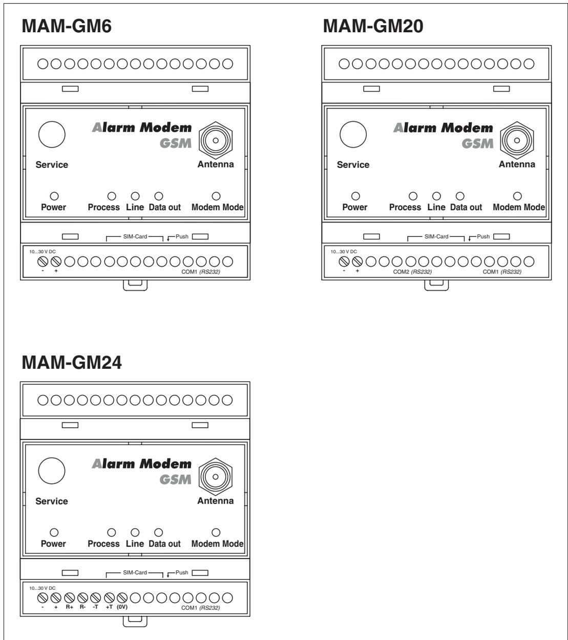
**Fig. 10-3:** MAM-GMx: Mitsubishi Alarm Modems GSM with RS232 and RS485
