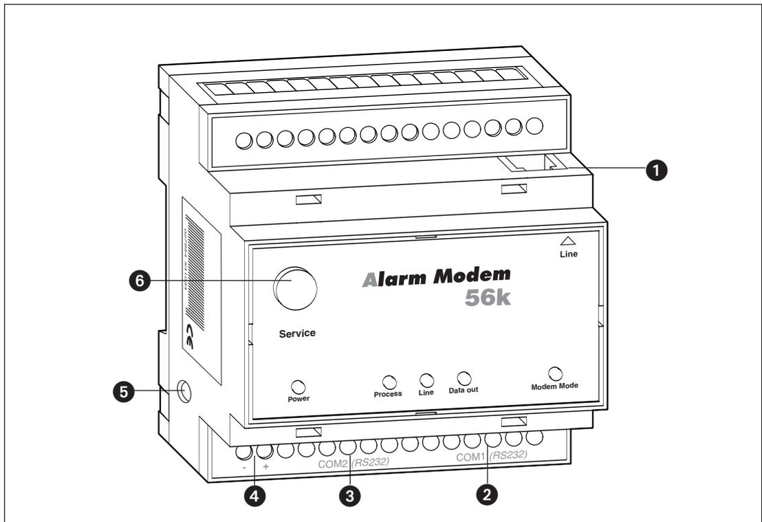
**Fig. 3-2:** Overview of all connectors of the Alarm Modem 56k
