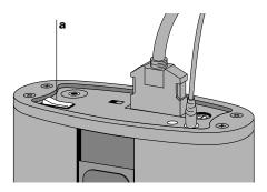
**2** Insert a small screwdriver into the slot of the SCSI ID selector on the camera and rotate the selector until the arrow points to the desired SCSI ID.
