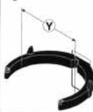
The bearing (A) has two diameters. As standard the mixer is delivered with the bearings mounted so that the smallest diameter points away from the bowl arms, which means the loosest bowl clamping.
