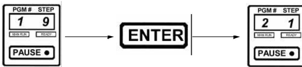
To edit a recipe or to correct mistakes, use the same step above to enter the programming mode, then push “ENTER” to reach the program/step that you wish to edit.
