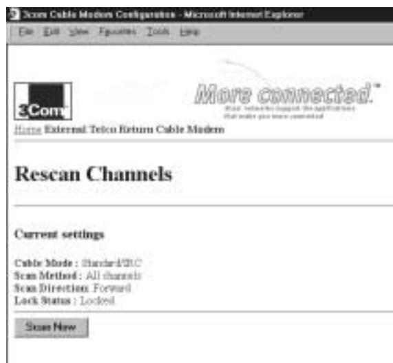
This menu allows you to manually start a scan for an open channel by clicking the **Scan Now** button. This is useful if for some reason the cable modem is not currently locked on to an active signal.
