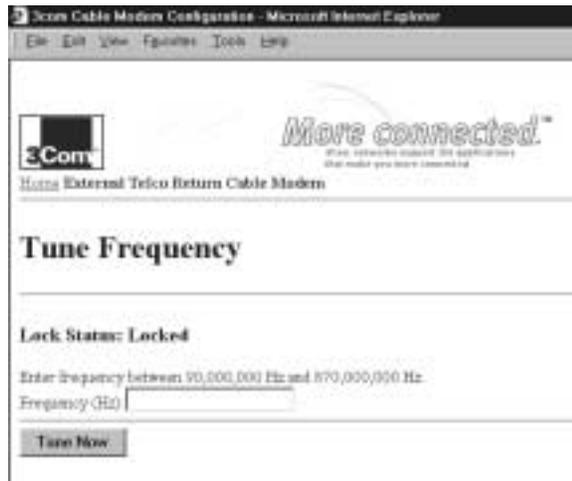
This screen allows you to tune the cable modem to an exact frequency. Type the frequency you want to tune to in the "Frequency (Hz)" box and then click **Tune Now** to set the modem to that frequency.
