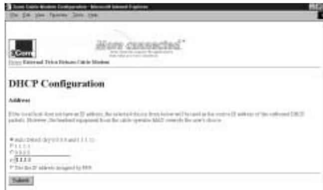
This screen allows you to select options for detecting/selecting source IP addresses for out-bound DHCP packets. Choose your method of detection and then click **Submit**.
