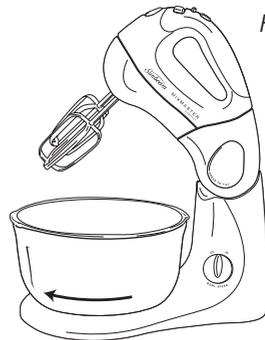
5. To lower the head of the mixer and beaters/dough hooks into the bowl, depress the 'tilt' button, hold the handle with the other hand and ease the head of the mixer down. A 'click' will indicate when the head has reached the correct position, see figure 4 over page.
