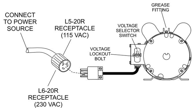
**Figure 7. Single Phase Electric Motor With 12-inch Pigtail**
