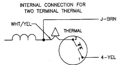
**Figure 38. Electric Motor Wiring Diagram**
