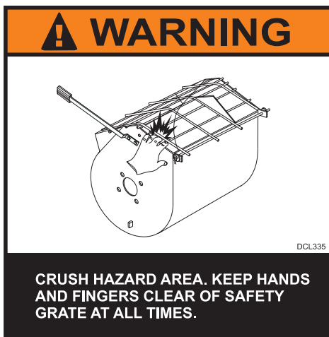
Figure 38. Safety Grate (Crush Hazard)
