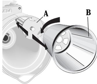
Attach shaft (A) to desired cone (B). Insert square end of shaft in square opening of housing and tighten by turning cone clockwise. Reverse to remove. Insert the cone assembly into housing (C) so shaft fits into square attachment hub socket. As you insert the cone assembly, lift up on the latch (D) and turn the cone assembly until it fits squarely in the attachment hub.
