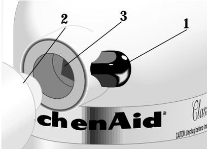
Before attaching accessory, turn off and unplug unit. Loosen attachment knob (1) by turning it counterclockwise. Remove attachment hub cover. Insert attachment shaft housing (2) into attachment hub (3) making certain that attachment power shaft fits into square hub socket. Rotate attachment back and forth if necessary. When attachment is in proper position, the pin on the attachment will fit into the notch on the hub rim. Tighten attachment knob until attachment is completely secured to mixer.
