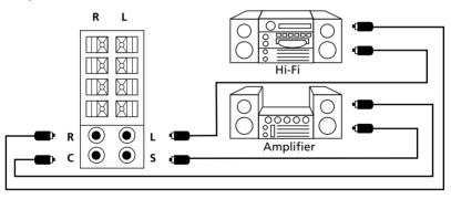
Dummy plug : Cut the sound from the internal loudspeaker
