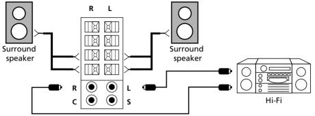
After making the connection, choose **configuration 4** from the **SPEAKER CONFIGURATION** menu, and **Dolby** from the **LOUDSPEAKERS** menu.
