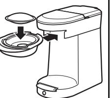
7. After you have finished your coffee and the coffeemaker has cooled, use the tab on the front of the brew basket to slide out brew basket and dispose of pod(s). If using standard tea bags, follow all directions except in step 2, remove brew basket and brew water directly into cup. Once hot water is brewed, steep tea bag in cup until desired strength is reached.
