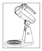
To tilt the mixing head, upward, press the head lock button inward while pulling up on the handle of the mixing head.
