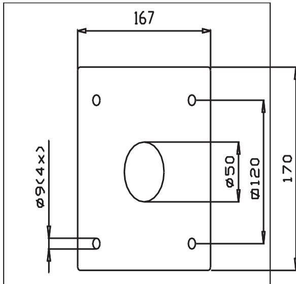
The foot plate of the GraviMaster should be attached on a steel attachment plate on the frame or mezzanine or flange pertinent to the machine.
