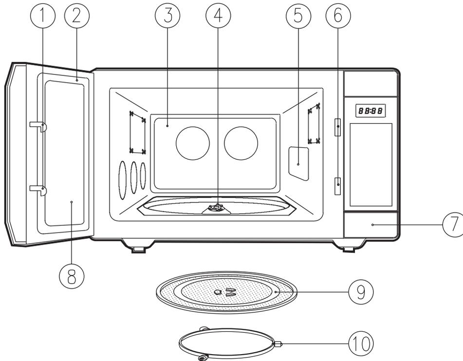
① **Door latch** - When the door is closed, it will automatically shut off. If the door is opened while the oven is operating, the magnetron will automatically shut off.
