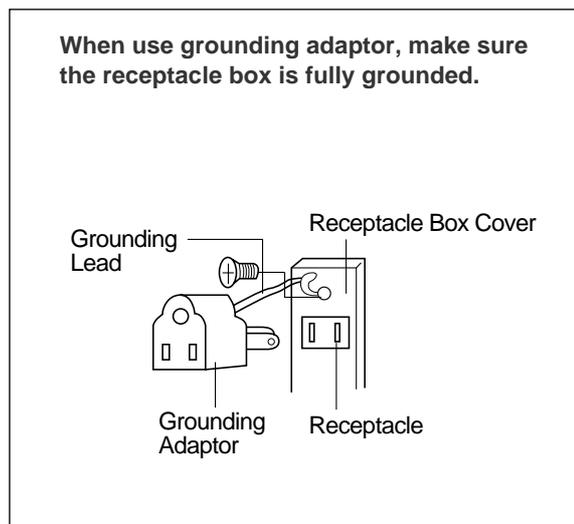
“THE CANADIAN ELECTRICAL CODE DOES NOT ALLOW THE USE OF THE GROUNDING ADAPTOR”
