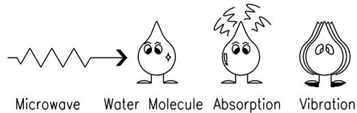
The microwaves cause the water molecules to vibrate which causes **FRICTION**, i.e. **HEAT**. This heat then cooks the food. Microwaves are also attracted to fat and sugar particles, and foods high in these will cook more quickly. Microwaves can only penetrate to a depth of 1 1/2 - 2 inches(4-5cm) and as heat spreads through the food by conduction, just as in a traditional oven, the food cooks from the outside inwards.
