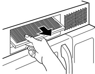
5. **Slide** a new charcoal filter into place. The filter should rest at the angle shown.
