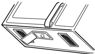
2. **Remove** the bulb cover mounting screws.
