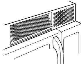
6. **Slide** the bottom of the vent grille into place. **Push** the top until it snaps into place. **Replace** the mounting screws.
