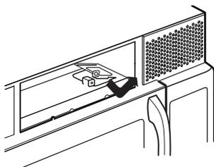
6. **Replace** bulb with a 30 or 40 watt appliance bulb.
