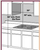
Each Sharp Over the Range microwave oven can be easily adapted for either outside ventilation (vertical or horizontal) or non-vented, ductless recirculation. Make sure the top of oven will be at least 66" from the floor and at least 30" from the cooking surface. A separate 15 amp. or greater electrical receptacle must be located in the cabinet directly above the microwave oven.
