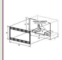
Your Sharp Microwave Oven can be built into your kitchen wall or cabinet using the appropriate Sharp Built-in Kit. Complete hardware and easy-to-follow instructions are included. Prepare cabinet or wall opening according to the illustration at left, providing access to a separate 3-pronged, 120V AC outlet, 15 amps. or larger.
